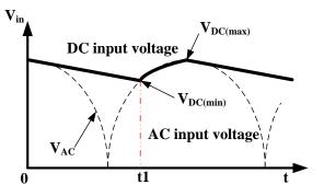
Figure 6: Input voltage waveform
