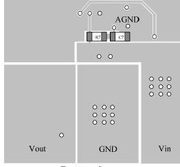
Bottom Layer Figure 15—PCB Layout
