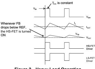
Figure 2—Heavy Load Operation
