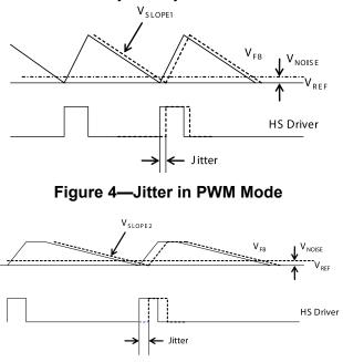
Figure 5—Jitter in Skip Mode
