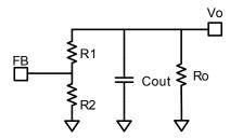
Figure 8—Simplified Circuit in skip Mode
