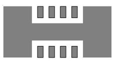
(e) Copper Area =  $70 \text{ mm}^2$ ,  $\theta_{\text{JA}} = 49^{\circ} \text{C/W}$
