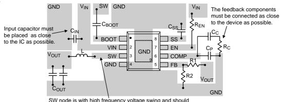
SW node is with high frequency voltage swing and should be kept at small area. Keep analog components away from the SW node to prevent stray capacitive noise pick-up
