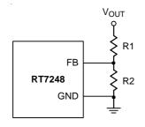
Figure 1. Output Voltage Setting
