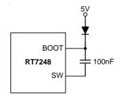
Figure 2. External Bootstrap Diode
