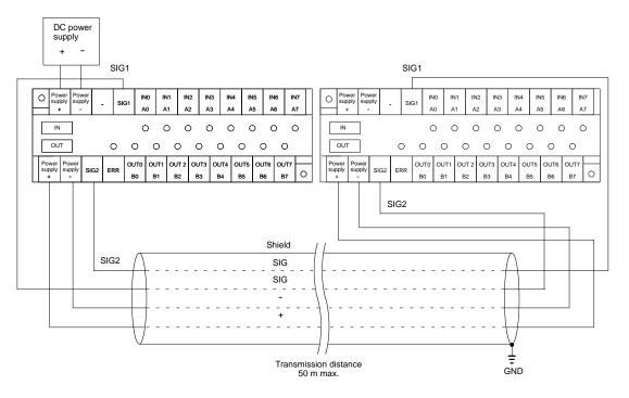
Note: In this example, a shielded transmission cable with a thickness of 0.75 mm<sup>2</sup> min. is used, through which a current of 1.8 A max. can be transmitted. It is recommended that the shield be grounded.
