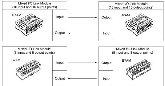
Note: The Mixed I/O Link Terminals are either 3 ms (typical, for high-speed models) or 19.2 ms (typical, for normal-speed models). Use a combination of an Input and an Output Link Terminal with the same transmission speed (I/O delay time).
