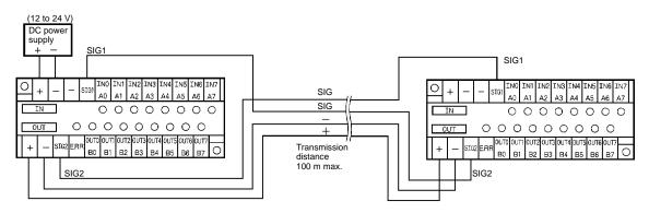
Note: In this example, a twisted pair or VCTF transmission cable with a thickness of 0.75 mm<sup>2</sup> min. is used, through which a current of 1.8 A max. can be transmitted.
