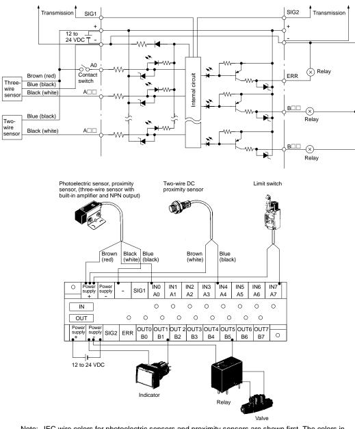
Note: IEC wire colors for photoelectric sensors and proximity sensors are shown first. The colors in parentheses refer to the old colors.
