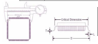
\* To calculate the "Critical Dimension" refer to manufacture data sheet or measure with calipers to determine the nominal value of "D", "L" and "T".
