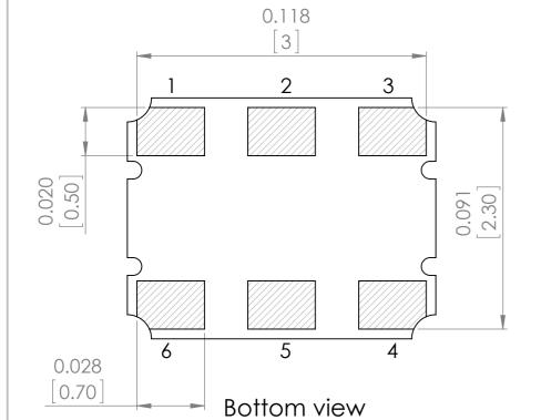
Note1: It is the Recommended To use approximately 0.01 uFby pass capacitor between PIN 3 and 6.
