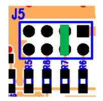
Figure 2: Output Voltage selection jumpers J5. Nominal jumper position voltages from left to right are: 3.31V, 1.8V, 1.2V and 1.0V. Jumper shown selects 1.20V output. Do not change jumper positions while the board is powered.
