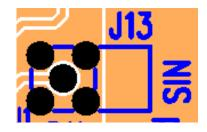
Figure 3: SMA Connector for External Clock Input
