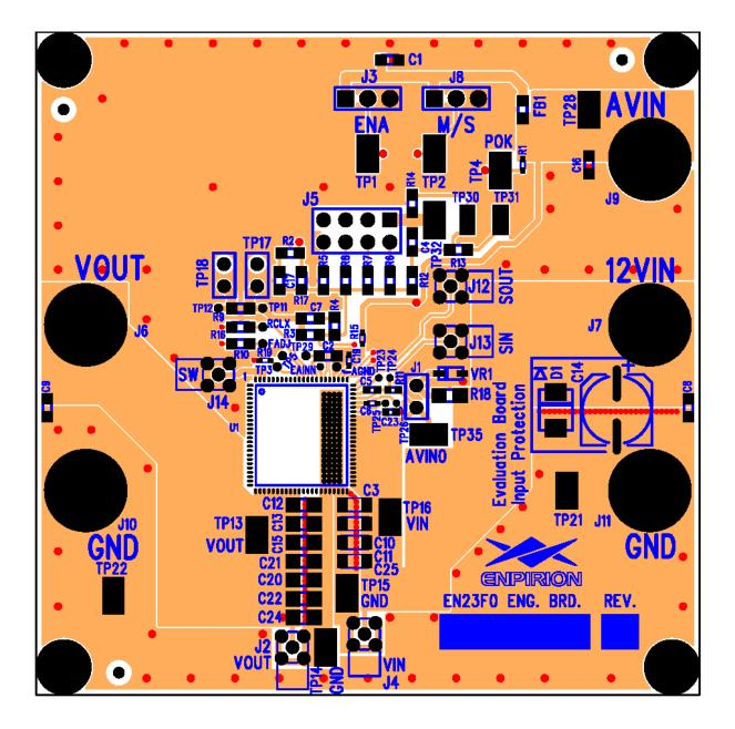
Figure 4: Evaluation Board Top and Assembly Layers.
